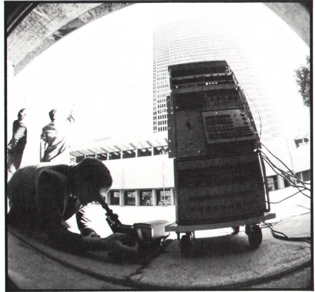
Fig. 8. Another vibration measurement using the interferometer and the Fourier analyzer. This one measured the resonances of a large office building.
